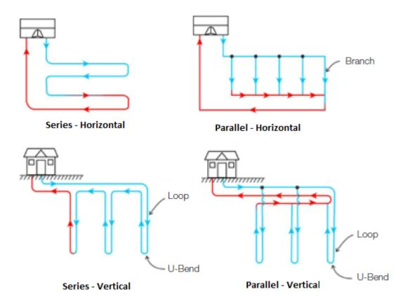
The type of arrangement will influence the pipe diameter, pump power requirements and installation cost. Advantages and disadvantages of series and parallel arrangements are summarized below.
