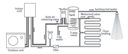
In colder climates, an antifreeze solution is circulated between the outside unit and indoor load. This reduces the risk of freezing during a power outage or if the heat pump becomes inoperable during cold weather. The antifreeze solution can be directly circulated through the indoor distribution system or separated from a water-based hydronic distribution system using a heat exchanger, as shown in the Figure below.
