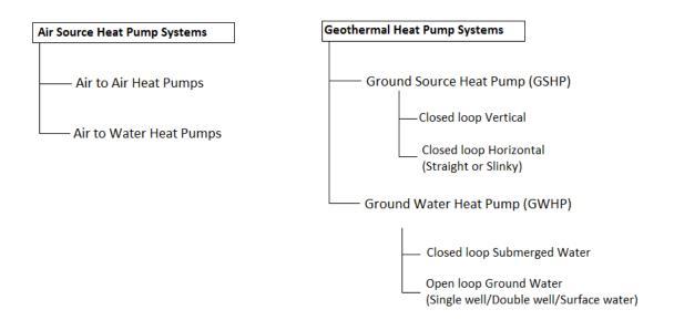
How these systems are adapted to building structures depends on the used application and source of energy. We will discuss the most common heat pump applications in next chapter.
