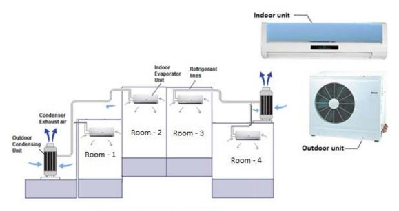
FREE DISCHARGE SPLIT UNIT HEAT PUMPS (COOLING CYCLE)
