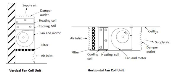
Hot water produced in the heat pump at a temperature of 120°F is pumped through the heating coil. The heating coil is generally 2 rows deep.
