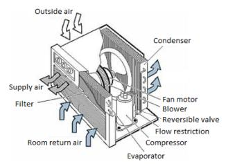
While a customer will typically select the window heat pump unit based on the cooling capacity, it is also important to pay attention to the heating capacity. This will allow selecting the right size unit for installation in a colder climate. Refer to the table below, indicating the comparison of two brands.
