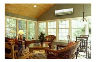
The typical range of capacities for these products is from 0.5 to 8 tons ( $\sim$ 1.75–28 kW) for a single split, and from 2 to 40 tons ( $\sim$ 7– 140 kW) for a multi-split unit.
