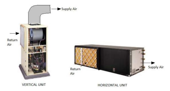
Packaged units contain an integral blower and a heat exchanger section that is connected to the air distribution system. Basic components used in the packaged equipment are the hermetic compressor, co-axial refrigerant-to-water exchanger, a finned coil refrigerant-to-air heat exchanger, a blower motor to circulate the air, and a capillary or refrigerant metering device. The system reverses from the cooling to heating cycles by means of a reversing valve.
