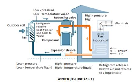
The outdoor unit fan draws air from open environment, which flows over the outdoor coil containing a refrigerant liquid. The liquid refrigerant absorbs the heat from the air and boils (evaporates) to vapor. The outside coil is thus referred to as Evaporator.
