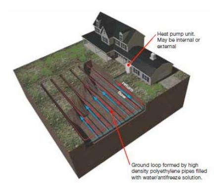
Horizontal loop system can be configured as straight, multiple or slinky arrangement.
