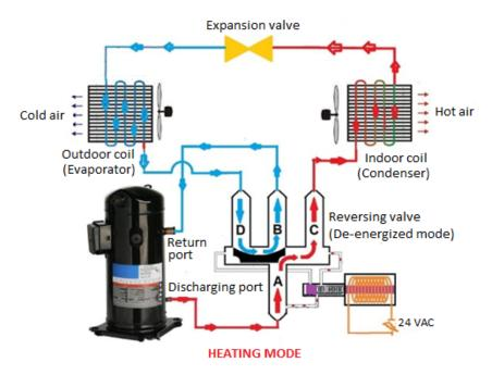
The outdoor coil of the heat pump will gather low-temperature heat from environment, where that heat is freely available and abundant (ground, water or air). The condenser side will always deliver higher temperature heat to the load.
