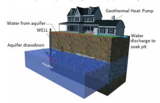
This system provides an economical solution if there is a preexisting well. In residential situations, a domestic water supply well could possibly be too small to meet the water needs of the groundwater heat pump. Residential wells typically produce 300 to 400 gallons of water per day, where a groundwater heat pump for the same residence may require thousands of gallons of water per day. A slightly modified single-well system which may alleviate some of these concerns is a standing-column well.
