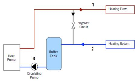
Incorporating a buffer tank into a heat pump system
