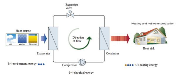
The key to the efficiency of a heat pump is the Coefficient of Performance: the "COP".
