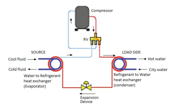
The load side provides hot water for use in bathrooms, laundry, and kitchen, as well as for pool heating or heating large areas in underfloor or wall-mounted heating systems.
