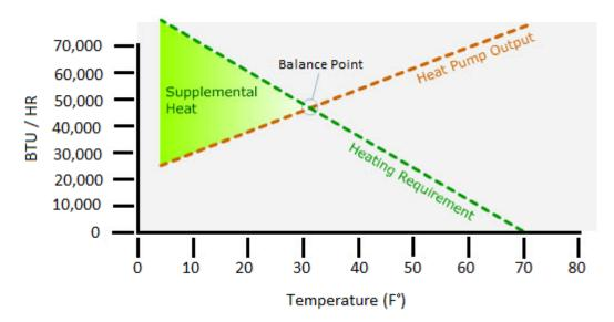
The supplementary heat can be supplied by an oil, gas or electric furnace or in the form of electric-resistance heaters. Supplementary heating is energized only when the space heating load cannot be met by the capacity of the heat pump. ASHRAE/IESNA Standard 90.1-1999 stipulates heat pumps equipped with internal electrical resistance heaters shall have controls to prevent supplemental heater operation when the heating load can be met by the heat pump alone during heating or setback recovery.
