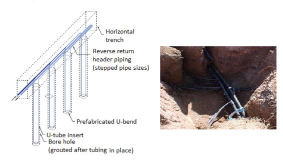
All earth loops, especially those with buried (inaccessible) fusion joints, should be pressure tested with compressed air to at least 75 psi for at least 24 hours to ensure there are absolutely no leaks.
