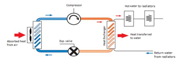
The air source heat pump does not produce the sort of hot water temperature you would associate with a gas, LPG or oil powered boiler. With a boiler, you would expect the hot water to be heated to about 185°F (85°C), while a heat pump produces water to about 130°F (~55°C). This means, greater volume of water will be needed to satisfy the heating requirements.
